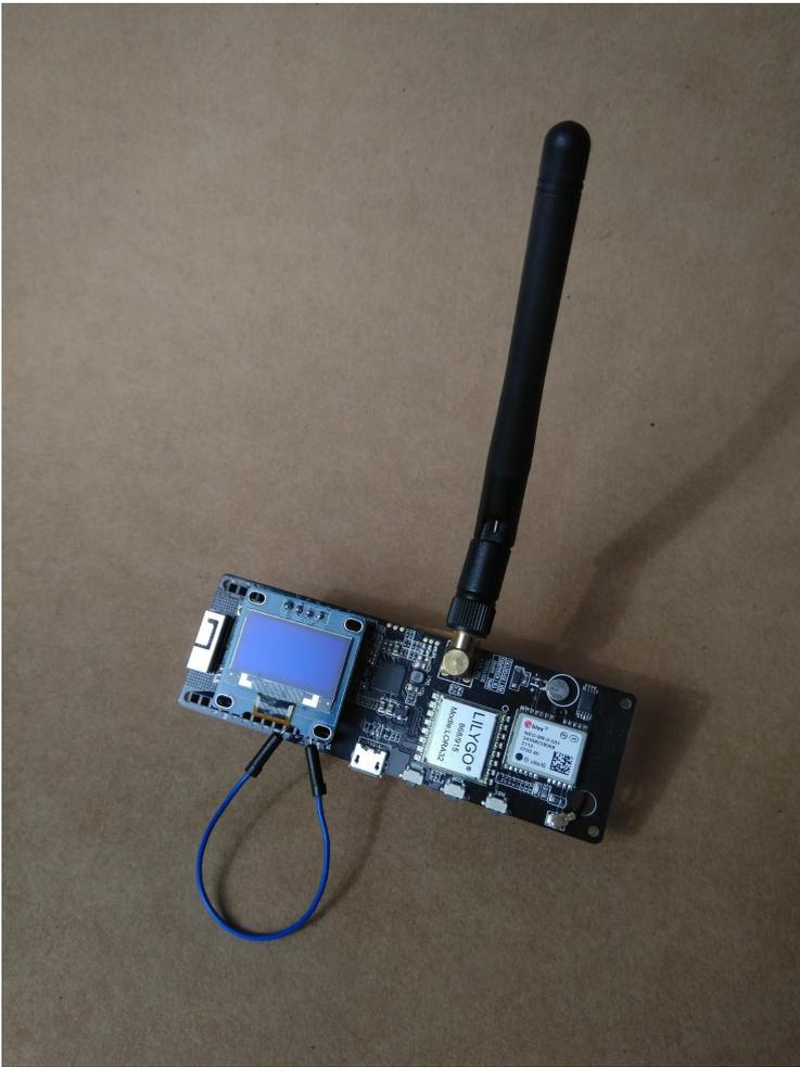
Pictured is an assembled demo device. The OLED display is visible on the left of the board. The LoRa antenna attaches to the top. The battery is attached underneath the board (not visible). The blue wire at the bottom of the board represents the switch to sense trap status.
